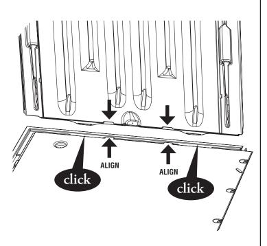
Hold Repeat Right Side (E) upright to prevent it from falling (until Right Back (F) is installed).
